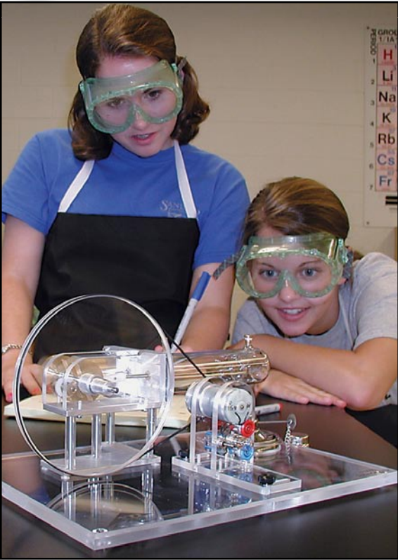
The Stirling engine includes a motor-generator and can be operated as a thermal engine, heat pump, and/or a refrigerator.
