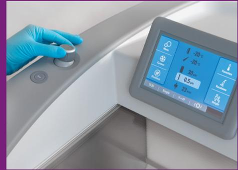
NX70 cryostats feature motorized sectioning for ease of use and to reduce the need for repetitive motions
