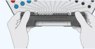
Use the Transfer Rack to lift Reaction Tubes from the Workflow Tray.
