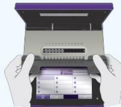
Release the Reaction Tubes from the Transfer Rack by pulling the Transfer Rack toward your body.
