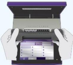
Lower the Reaction Tubes into Solana.
