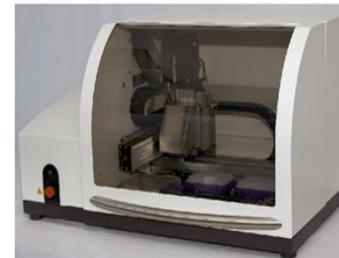
Open Array plate loading using the AccuFill system
