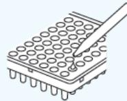
Add 5  $\mu$ L of sample with process control to plate well and seal the plate. Centrifuge plate for 15 seconds.
