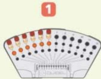
Setup the Workflow Tray with patient samples, Process Buffer Tubes and Reaction Tubes.
