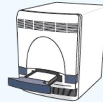
Insert plate into 7500 Fast Dx or
