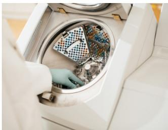
The automated tissue processor, **Epredia Revos**, used in this study, has a canted chamber, allows sufficient penetration of the process reagent into specimens repeatedly immersed and removed from the reagent solution.
