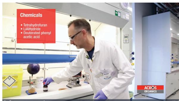
To get the best results from the septum, we recommend you use 18- to 21-gauge needles and puncture in a clock face pattern to avoid piercing the septum in the same place.
