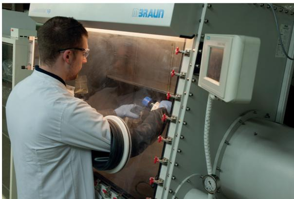
Glove box to handle air- and moisture-sensitive reagents
