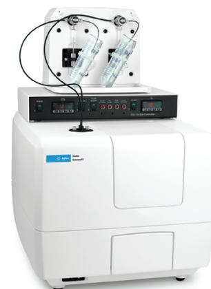
Synergy H1 shown with CO<sub>2</sub>/O<sub>2</sub> gas controller and dual reagent injector.
