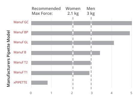
The graph on the left shows a comparison between traditional universal pipetting systems and the Biotix Ergonomix System. For this test we used a continuous insertion force of 5 kg averaged across three tip sizes. The positive stop built into the Ergonomix System keeps the ejection force below the recommended levels by ergonomists for both men and women. All competitors are above either the men or women recommended levels which can lead to increased fatigue and risk of RSI/RSD.
