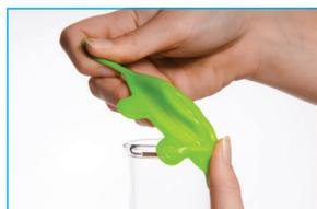
Position the edge of the vessel opening in the groove located on the inner surface of the lid.
