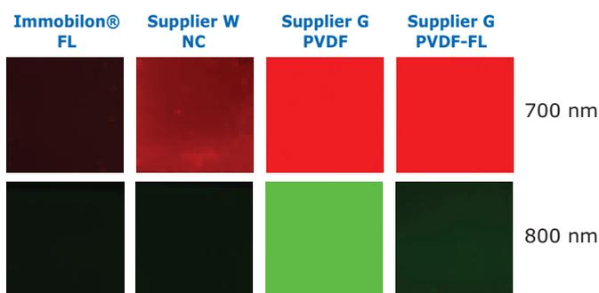
**Figure 15.** Comparison of background fluorescence observed in PVDF membranes from different manufacturers. Only Immobilon®-FL membrane offers low background fluorescence at both 700 and 800 nm, increasing its ability to be used in multiple excitation and emission wavelengths.
