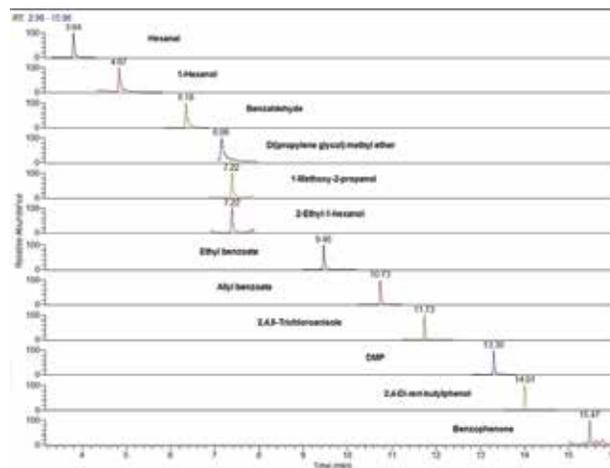
Figure 4. Chromatogram of spiked paperboard with 12 packaging migrants (c = 0.024–30 mg/kg)
