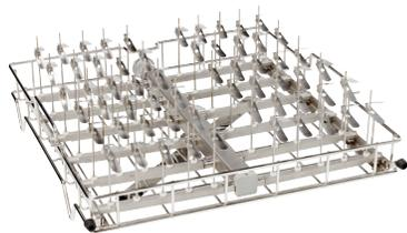
**Upper Small Spindle Racks.** High-capacity design provides 60 spindles, 60 adjustable height clips, 60 spindle plugs, 12 spindle arm plugs, spindle tool and wash arm for cleaning of small narrow-neck glassware. 304 stainless steel. Spindle dimensions: 4.4" h x 0.125" OD. Overall dimensions: 21.5" w x 20.8" d x 7.3" h. Accommodate glassware up to 8.9" h.
