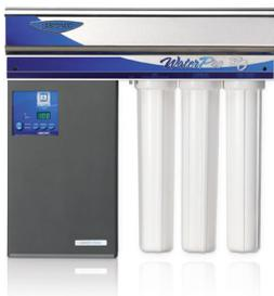
**WaterPro® RO Systems.** Connect to Labconco glassware washers to provide purified water for the rinse cycles. Deliver 1 L/min of reverse osmosis purified, Type III water when feedwater purity is 100 µs or better.
