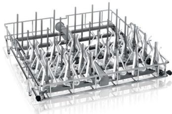
**Upper Spindle Racks.** 304 stainless steel. Includes 36 removable spindles, 36 adjustable height clips, 18 plastic glassware holders, 10 small spindles with clips, 36 spindle plugs, 12 spindle arm plugs and wash arm. Spindles or spindle arms may be removed and plugged to accommodate accessory inserts (sold separately). Spindle dimensions: 4.5" h x 0.25" OD. Overall dimensions: 20.8" w x 21.6" d x 6.9" h. Accommodate glassware up to 8.9" h.
