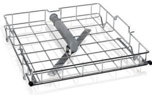
**Upper Standard Racks.** One is included with every SteamScrubber. May be used in any FlaskScrubber or FlaskScrubber Vantage. 304 stainless steel. Includes side release latches and wash arm. Add accessory inserts to suit your glassware mix (sold separately). Overall dimensions: 21.5" w x 20.8" d x 6.0" h.
