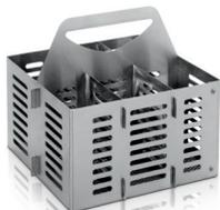
**15-352-014—Utensil Holder.** For spatulas, spoons, scoops and other miscellaneous utensils. Utensils fit vertically in six compartments, 2.6" w x 4.4" d x 4.9" h. 304 stainless steel. Overall dimensions: 8.2" w x 8.2" d x 8.0" h. For use in Upper or Lower Standard or Spindle Racks. Shipping weight 5.0 lbs. (2.3 kg)
