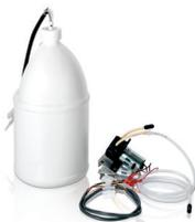
**15-352-020—Liquid Detergent Dispenser Kit.** Connects to any FlaskScrubber or SteamScrubber to automate liquid detergent dispensing. Includes peristaltic pump, float switch, tubing and one gallon plastic container. **Detergent required (not included).** Shipping weight 3.0 lbs. (1.4 kg)
