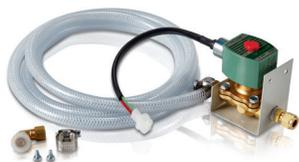
**Drain Water Cooling Kits.** Provide plumbing components, solenoid valve and electrical connections necessary to reduce drain water temperature to <math><140^{\circ}\text{F}</math> (<math><60^{\circ}\text{C}</math>). When the washer's drainage pump is activated, the solenoid valve opens, releasing the flow of cold tap water to the drain. Requires cold water connection. For use with any FlaskScrubber, SteamScrubber or FlaskScrubber Vantage. Shipping weight 6.0 lbs. (2.7 kg)
