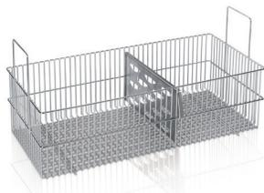
**15-352-003—Bulk Tube Insert.** Quick-loading design holds up to 600 each 13 mm tubes or 244 each 20 mm tubes. Divider securely holds tubes during wash cycle. Overall dimensions: 8.6" w x 17.7" d x 8.4" h. May use up to two per rack at one time. For use in Upper or Lower Standard or Spindle Racks. Shipping weight 6.0 lbs (2.7 kg)
