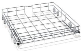
**15-352-039—Lower Standard Rack.** One is included with every SteamScrubber. May be used in place of Lower Spindle Rack in any FlaskScrubber or FlaskScrubber Vantage. 304 stainless steel. Add accessory inserts to suit your glassware mix (sold separately). Overall dimensions: 21.4" w x 20.9" d x 3.5" h. Shipping weight 12 lbs. (5 kg)
