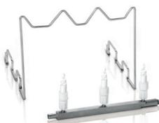
**15-352-009—Graduated Cylinder Insert.** Holds up to three graduated cylinders, each 1L or smaller. Includes three full-coverage spray nozzles for maximum cleanability. 304 stainless steel. May use up to two inserts per rack at one time. **For use with Lower Spindle Rack 4668900 (required, not included).** Overall dimensions: 7.6" w x 9.2" d x 10.0" h. Shipping weight 2.0 lbs. (0.9 kg)
