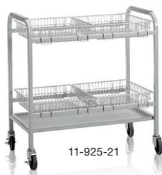
**Glassware Carts.** Safely transport clean and dirty labware. Come with two large or four small interchangeable vinyl-coated wire baskets and removable drip pan below the baskets to catch spills. Include 4" diameter casters (two with toe locks). Frame is welded 1" square mar-resistant, powder-coated tubular steel. Overall dimensions: 34.9" w x 19.0" d x 36.4" h. Fully assembled. Lifetime warranty. Shipping weight 43 lbs. (20 kg)
