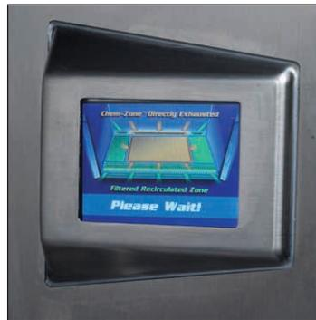
zone, there is no recirculation of air. In the ducted Type B mode, the Chem-Zone safely removes all chemical vapors generated above the dish, guaranteeing operator and laboratory safety. Air outside the zone—downflow air at the ends of the work surface and air taken in at the front grille—is recirculated to save energy in ducted applications. Table 1 below outlines the lifetime savings achieved by the Axiom Type C1
