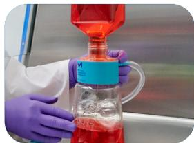
Stericup® E and Steritop® E filters thread directly onto any commercial media bottle or glass bottle:
