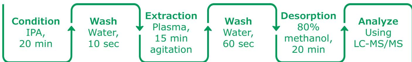
**Figure 1** Overview of the steps for the Supel™ BioSPME workflow in the determination of free fraction of drug in plasma.
