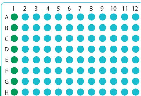
**Figure 6.** Overview of the “8 + 88 method”. Column 1 (green) contains spiked buffer sample and columns 2 – 12 contains the spiked plasma (blue). The buffer at the beginning of each row was used to calculate the %protein binding across that row (ex. Buffer A1 was used to calculate the %protein binding associated with wells A2 - A12).
