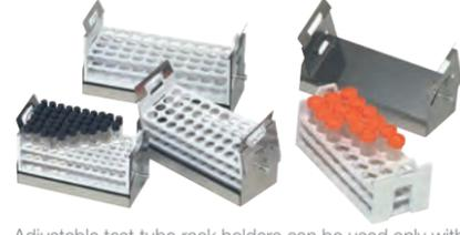
Adjustable test tube rack holders can be used only with their corresponding rack size. This design includes one test tube rack each.
