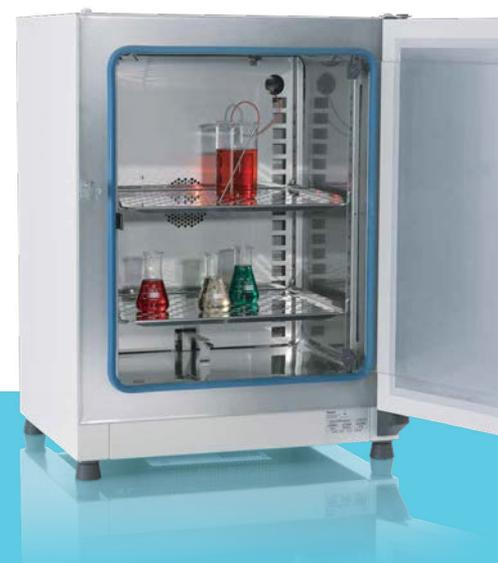
Heratherm Advanced Protocol Security microbiological incubator with unique dual convection and additional alarm systems, 100 L unit pictured
