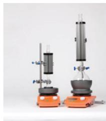
**Super Air Condenser** replaces the need for water cooled condenser in over 95% of all common chemistry applications
