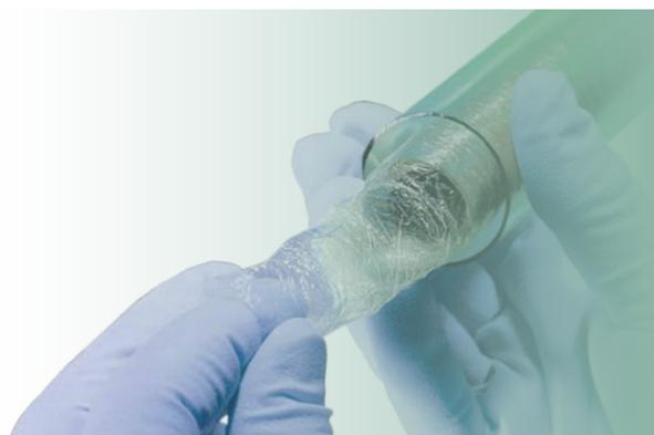
Thermo Scientific™ SnakeSkin™ Dialysis Tubing is an easy- and ready-to-use form of traditional dialysis membrane tubing that allows desalting and buffer exchange for 10 to 100 mL samples, and it does not require presoaking or boiling prior to use. To use, simply pull out and cut off the required length of tubing, fold over one end of tubing and close with a dialysis clip, add sample at the open end, and use a second clip to close the remaining end.
