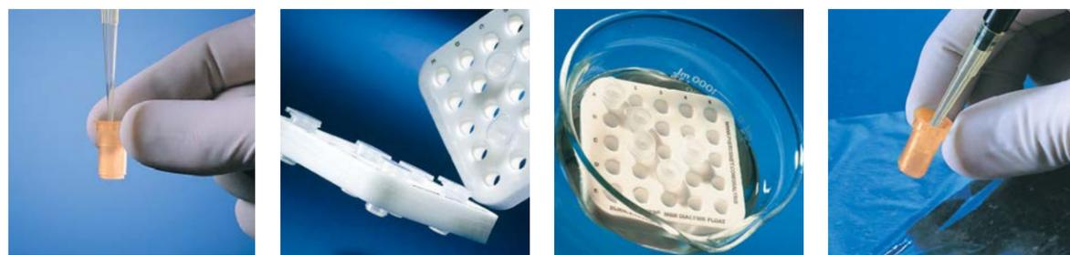
Figure 6. Sample dialysis using a 0.1 mL Thermo Scientific Slide-A-Lyzer MINI Dialysis Device. The required float is sold separately.
