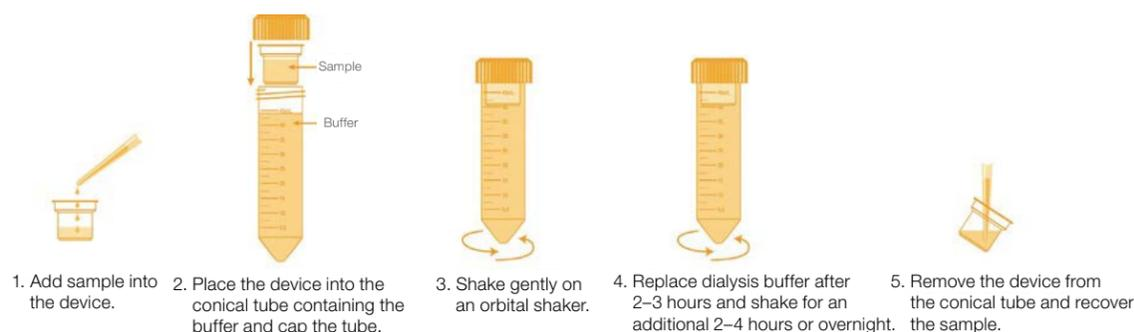
Figure 7. Sample dialysis with a 0.5 mL or 2 mL Thermo Scientific Slide-A-Lyzer MINI Dialysis Device.
