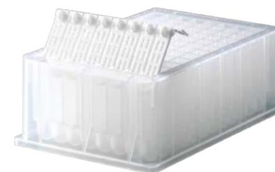
The Thermo Scientific Pierce 96-well Microdialysis Plate is an automation-compatible system for simultaneously dialyzing between 1 and 96 samples with volumes from 10 µL to 100 µL. The dialysis inserts are provided in strips of eight preloaded in a 96-well deep-well plate, but can be separated easily for use as individual dialysis devices in a standard microcentrifuge tube.
