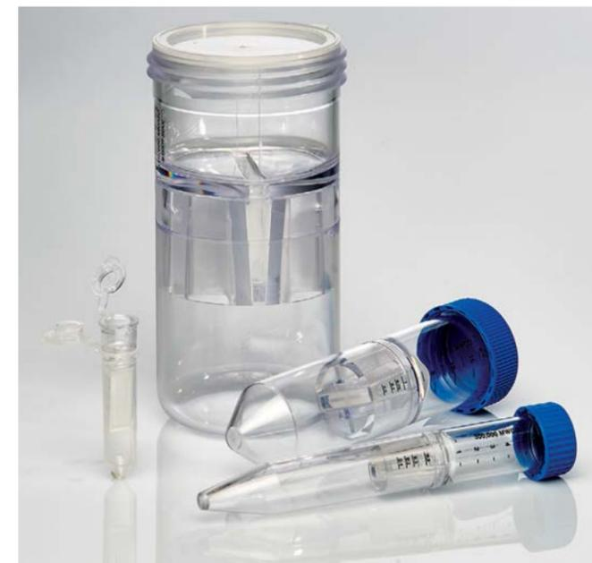
The most commonly used membranes for protein concentration devices are polyethersulfone (PES), regenerated cellulose, and cellulose triacetate (CTA). PES has a uniform surface devoid of hydrophobic or hydrophilic interactions and offers excellent protein recovery for most solutions. PES membranes exhibit
