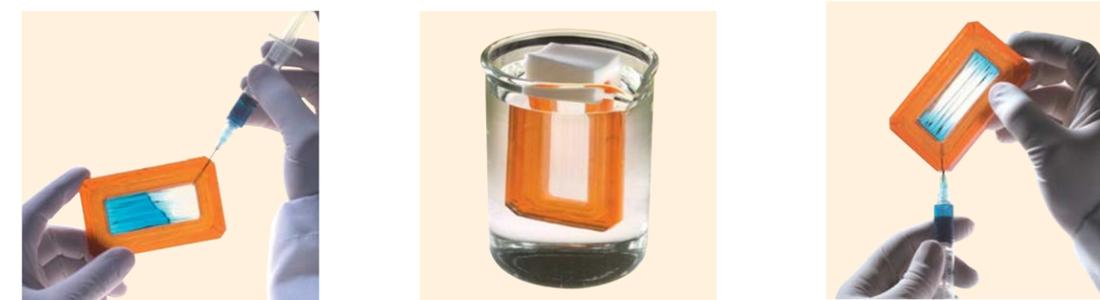
Figure 8. Thermo Scientific Slide-A-Lyzer Dialysis Cassette procedure summary.
