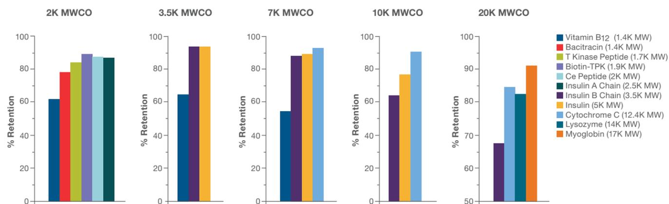
**Figure 3. Sample retention by the 2K, 3.5K, 7K, 10K and 20K MWCO Thermo Scientific Slide-A-Lyzer Dialysis Cassette membrane.** Individual proteins (1 mg/mL) in either saline or 0.2 M carbonate-bicarbonate buffer, pH 9.4 were dialyzed overnight (17 hours) at 4°C. The amount of retentate was estimated using either the Thermo Scientific™ Pierce™ BCA Protein Assay or absorption at 360 nm (for vitamin B12).
