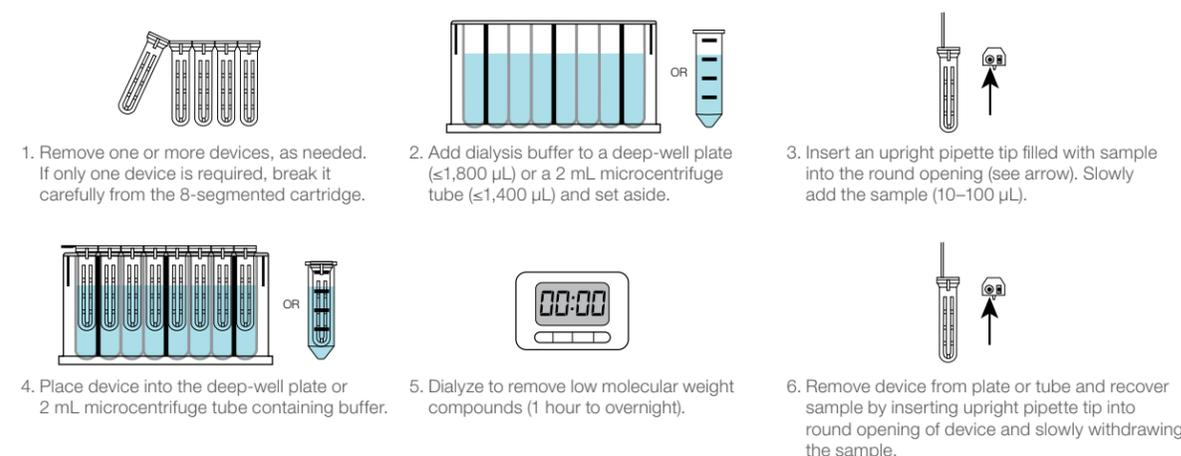
Figure 5. Protocol summary for the Thermo Scientific Pierce 96-well Microdialysis Plate.
