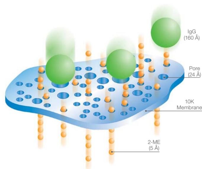
**Figure 1. How dialysis membranes work.** A dialysis membrane is a semi-permeable film (usually a sheet of regenerated cellulose) containing various sized pores. Molecules larger than the pores cannot pass through the membrane, but small molecules can do so freely. In this manner, dialysis may be used to perform purification or buffer exchange for samples containing macromolecules.
