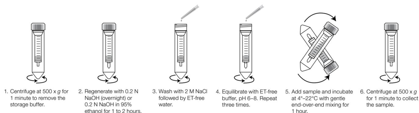
Figure 3. Protocol for Pierce High Capacity Endotoxin Removal Spin Columns.
