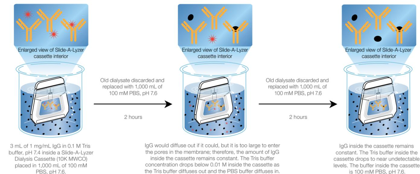
**Figure 2. How the Thermo Scientific Slide-A-Lyzer cassette works.**
