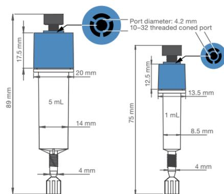
manually or by automated liquid chromatography (LC) systems. The cartridges attach directly to the ÄKTA™ FPLC™ system from GE Healthcare or other FPLC systems without additional connectors. Cartridge products include an accessory pack of tubing fittings and Luer-Lok™ fittings that provide compatibility with the other popular LC systems and manual syringe processing. They are available only in the 7K MWCO resin.
