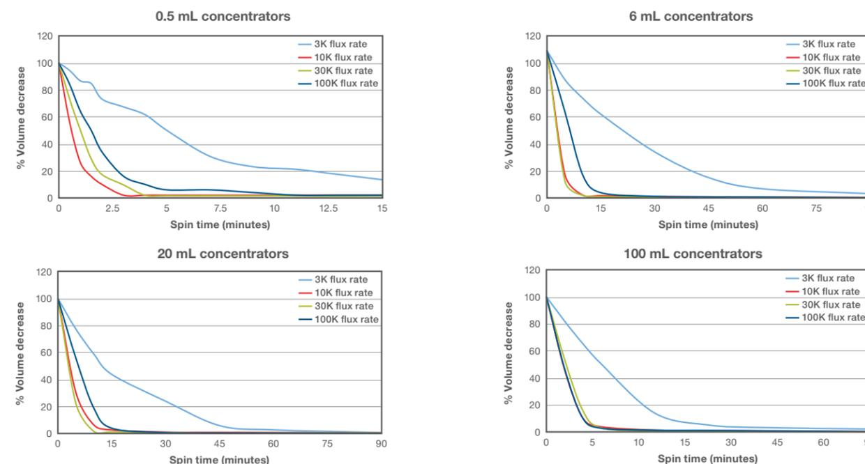
**Figure 4. Comparison of flux rates for different MWCOs using 0.5 mL, 6 mL, 20 mL, and 100 mL concentrators.** Samples of protein for each MWCO (Cytochrome C, 12 kDa (3K); Ovalbumin, 45 kDa (10K); BSA, 66 kDa (30K); and Thyroglobulin, 660 kDa (100K), at approximately 0.25 mg/mL starting concentrations) were centrifuged in Pierce Protein Concentrators to determine the rate at which >90% protein is concentrated.
