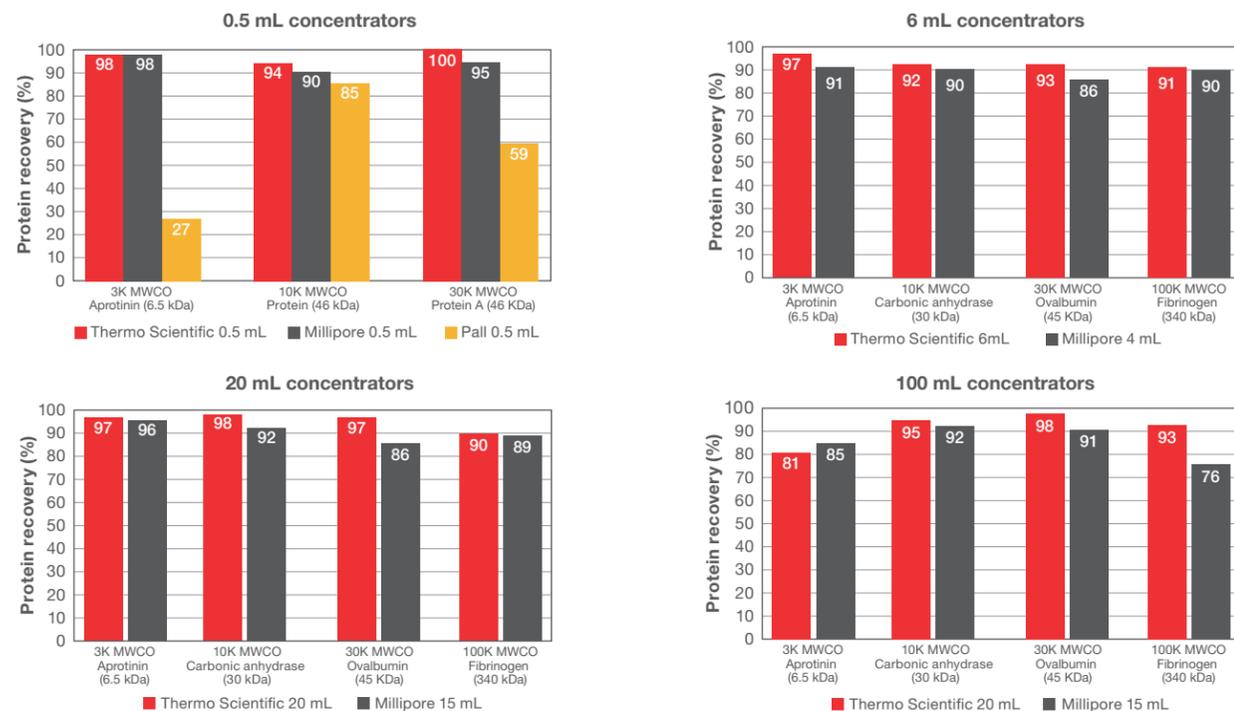
**Figure 2. Comparison of protein recovery between Pierce Concentrators (using 3K, 5K, 10K, 30K, or 100K MWCO) and other vendors for 0.5 mL, 6 mL, 20 mL, and 100 mL concentrators.** Samples of different protein solutions were centrifuged in Pierce Protein Concentrators and other suppliers' concentrators according to
