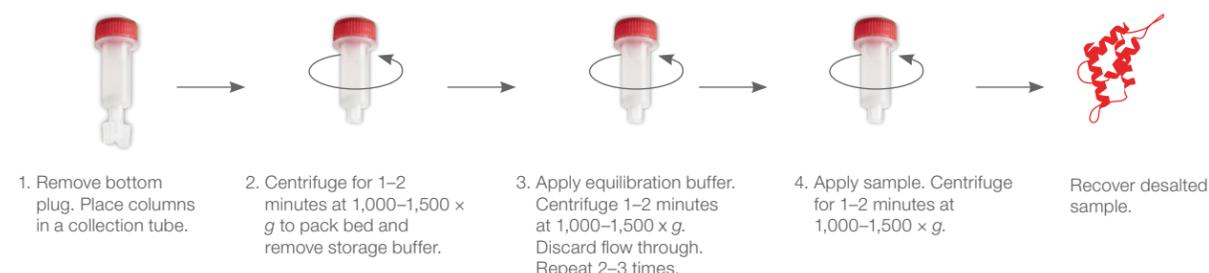
**Figure 2. Protocol for desalting with Thermo Scientific™ Zeba™ Spin Desalting Columns.**
