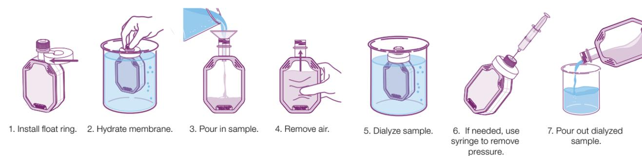
**Figure 10. Easy sample loading and recovery with Thermo Scientific Slide-A-Lyzer Dialysis Flasks.** Attach supplied float-ring and hydrate membrane for 2 minutes. Pour sample into device. Remove air and cap. Dialyze for 8 hours to overnight (replace buffer after 2 and 5 hours). Pour out sample to recover.
