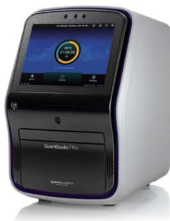
qPCR: Applied Biosystems QuantStudio 7 Pro Real-Time PCR System
