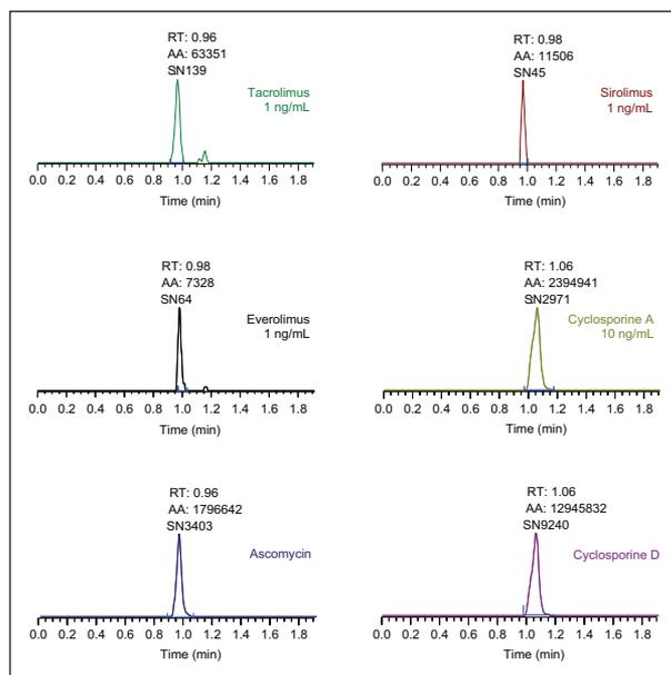
Figure 1. Extracted ion chromatograms with 5 ppm mass windows for analytes tacrolimus, sirolimus, everolimus (each at 1 ng/mL), and cyclosporine A (10 ng/mL), and internal standards ascomycin and cyclosporine D
