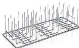
**48-Pin Insert** Securely holds smaller volume wide-mouth labware. Type 304 stainless steel with silicone tips to prevent scratching. For use in Labconco Upper or Lower, Standard or Spindle Rack. 10-Pin and 32-Pin Inserts also available. 8.5x18.5x4.5, 5 lbs., **15-352-008**
